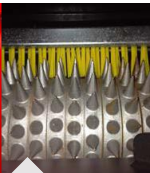
An optional brush scraper is available for the Speed-Seed to keep the spikes clean from soil build up.
