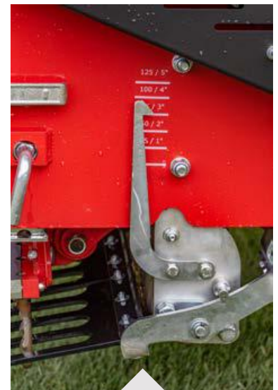
Manual Depth Control gives simple depth adjustment.
