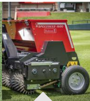
Adjustable gearbox for variable seed rates
