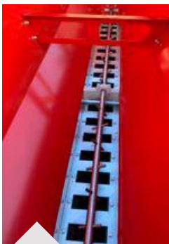
The accurate seed calibration system gives good distribution and less waste.
